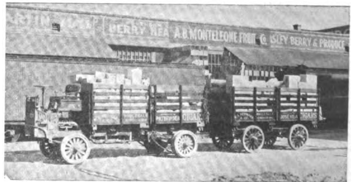
M. A. Newmark & Co., Los Angeles, Cal., made total deliveries of 20 to 25 tons a day with a five-ton truck. The use of a Troy Trailer raised their deliveries to 50 tons daily and divided the cost per ton.
